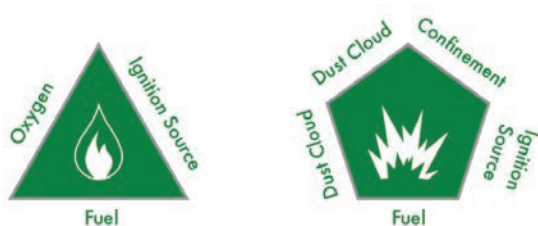
Figure 1. Fire triangle and explosion pentagon. Users of additive manufacturing are often working with fuel and oxygen, so ignition sources need to be avoided to prevent fires or explosions.
